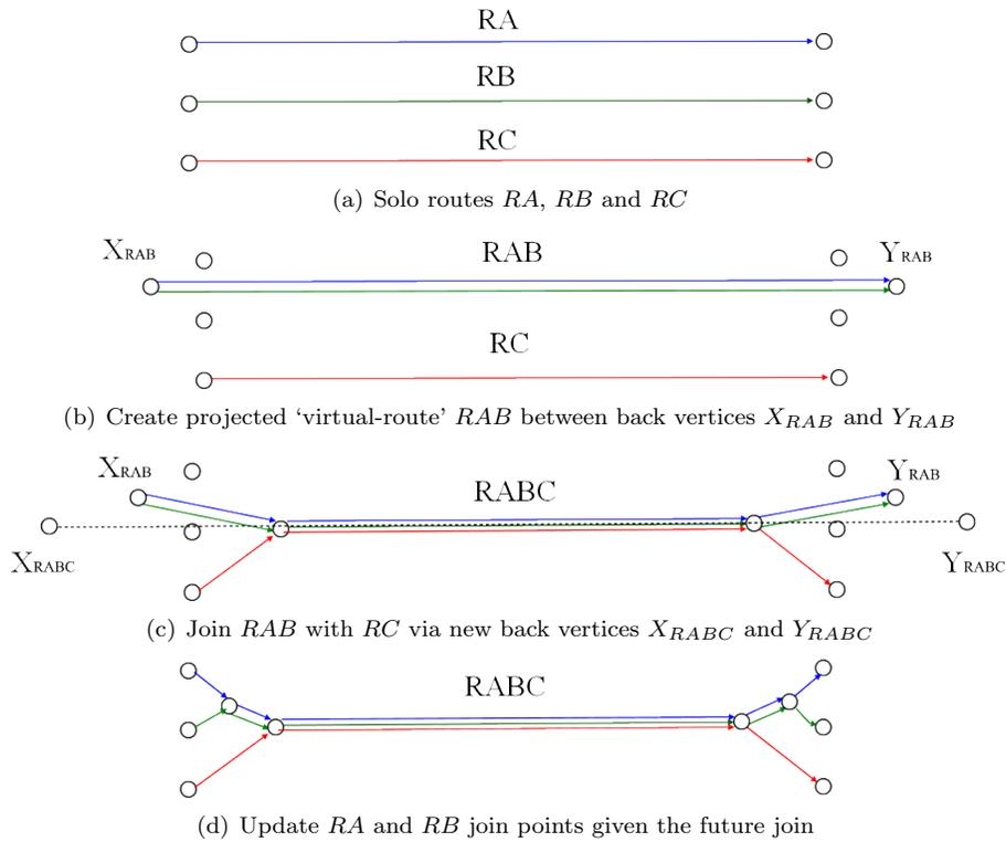
**Figure 5. Join and break points for three distinct routes**
