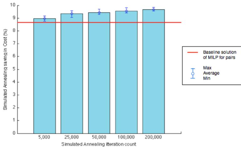
Figure 10. Percentage cost saving using formations of size three against solo flight
