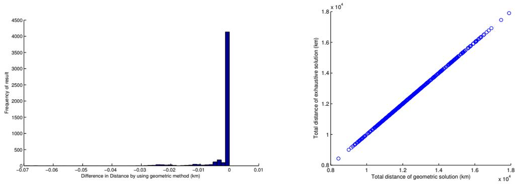
(a) Frequency in deviations between geometric solution and exhaustive search at 0.01 increments (b) Distances of geometric solution against exhaustive search
