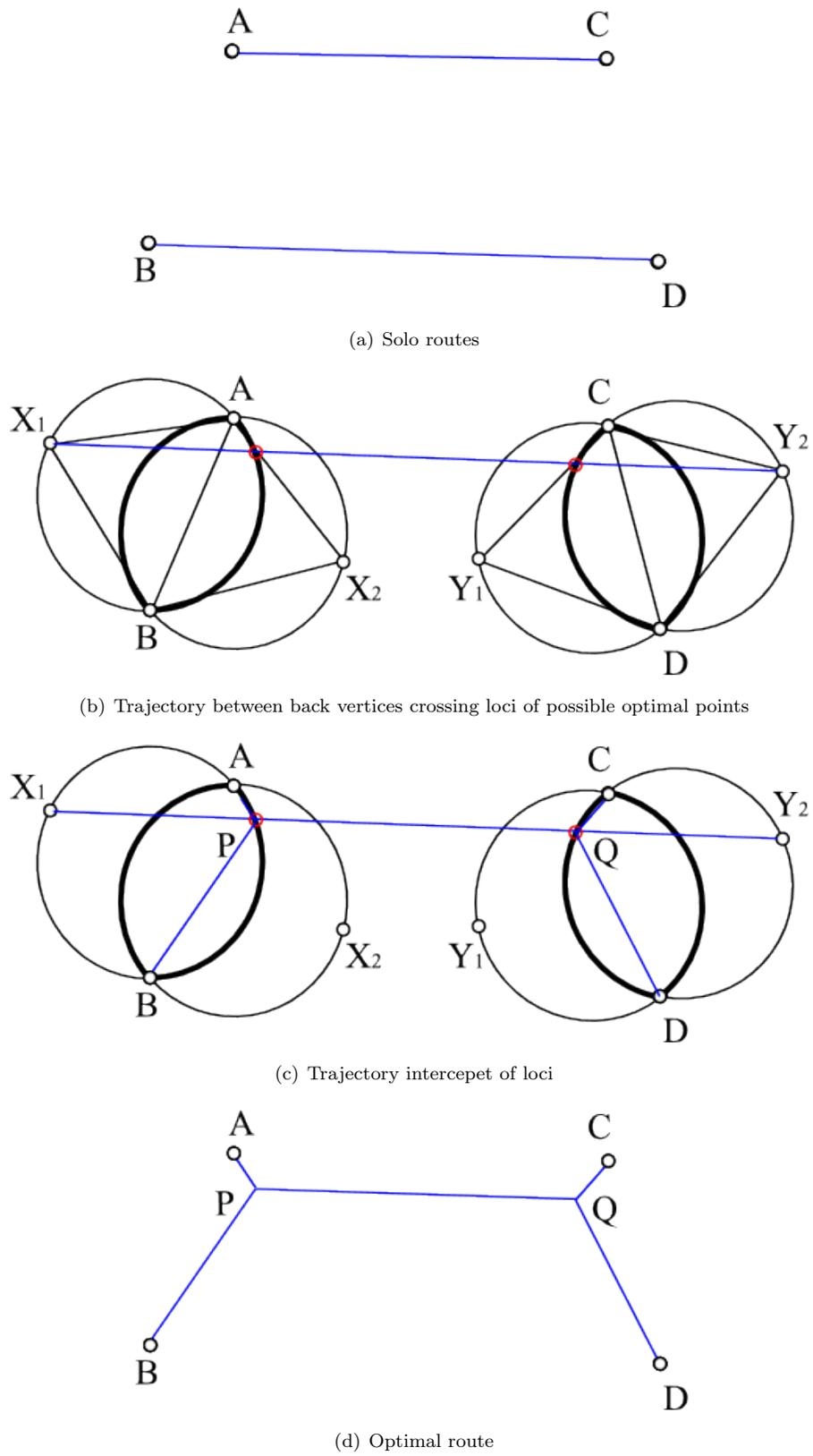
Figure 3. Join and break points for two distinct routes
