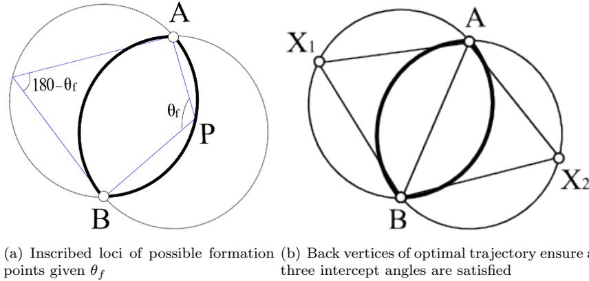
**Figure 2. Possible solution points given an angle of interception**
