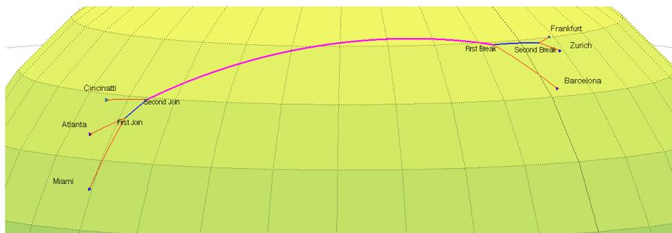
(b) Optimal formation route for the three routes *RouteA*, *RouteB* and *RouteC*
