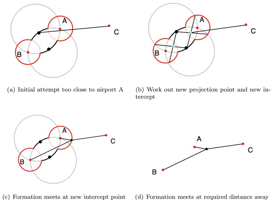
**Figure 7. New join point required to be at least a certain distance from each airport**
